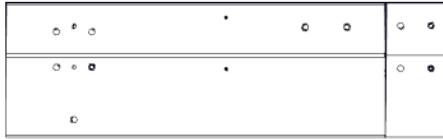
J04 JOIST ASSEMBLY - W2A03551 (x1) 1 7/16"x8 7/16"x28 7/16" (36x214x722)
