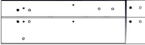
J01 JOIST ASSEMBLY - W2A03549 (x1) 1 7/16"x8 7/16"x28 7/16" (36x214x722)
