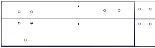
J01 JOIST ASSEMBLY - W2A03642 (x1) 1 7/16"x8 7/16"x28 7/16" (36x214x722)
