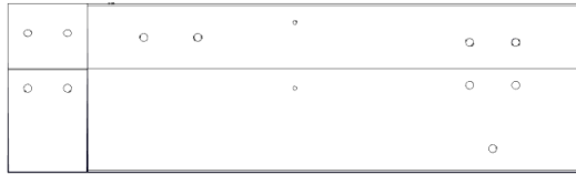
J03 JOIST ASSEMBLY - W2A03643 (x1) 1 7/16"x8 7/16"x28 7/16" (36x214x722)
