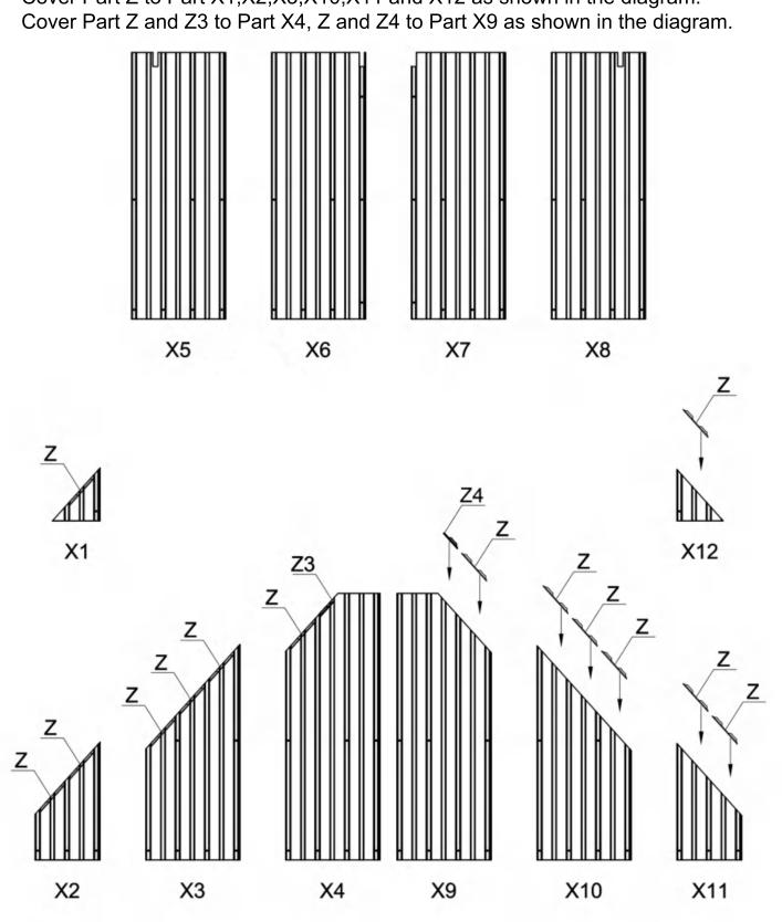
Overall Roof Assembly: Please put the panels on the frame anti-clockwisely.
