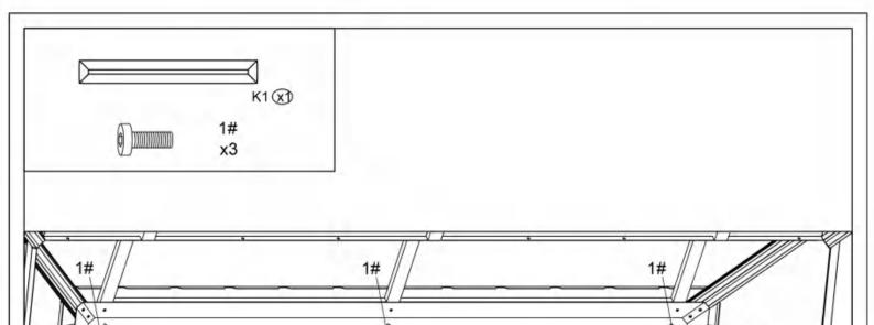
Step 10: Connect Part K1 (Outside Roof Connector) to Part K (Inside Roof Connector) using screw1#.
