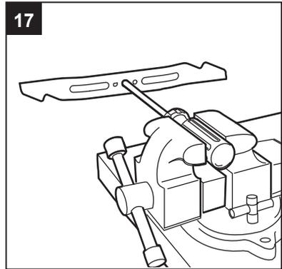
**NOTICE:** Keep the blade sharp for best mower performance. A dull blade does not cut grass cleanly or mulch properly.
