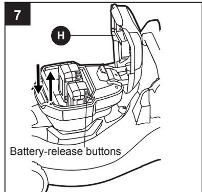
**NOTICE:** When placing the battery pack on the tool, be sure that the raised rib on the battery pack aligns with the groove on the tool and the latches snap into place properly. Improper assembly of the battery pack can cause damage to internal components.
